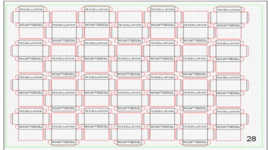
Above image shows 28 nets arranged for die cutting.
