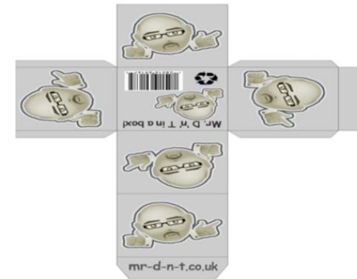
Remember the layout of text/images so they aren't upside down when assembled.
